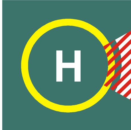
Figure 5-7. Helideck prohibited landing sector marking
